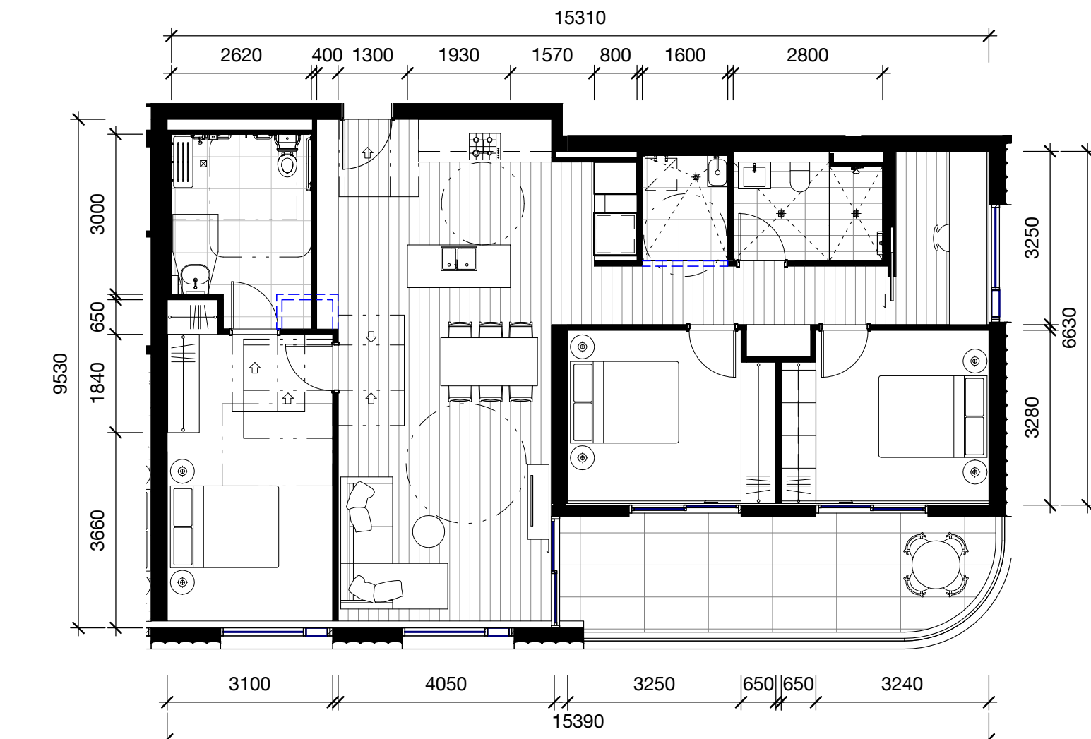
2 3 Bedroom Type A (Adapted) 1 : 100 Storage volume within apartment Storage cage in carpark Total storage volume compliant with SEPP65 guidelines (6.00m 2 )
